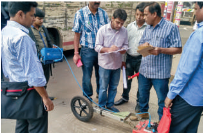
Ground Penetration Radar
