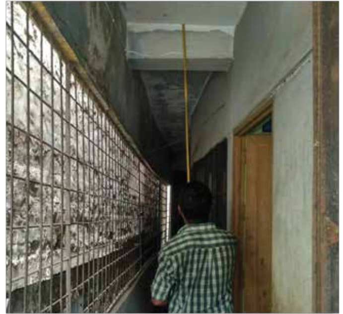
Data is being collected for As-built Drawing Preparation
