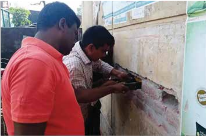
Brick Shear Strength Test on Masonry Structures
