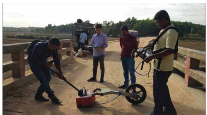
Team from BUET-JIDPUS performing the GPR scan on the slab bridge
