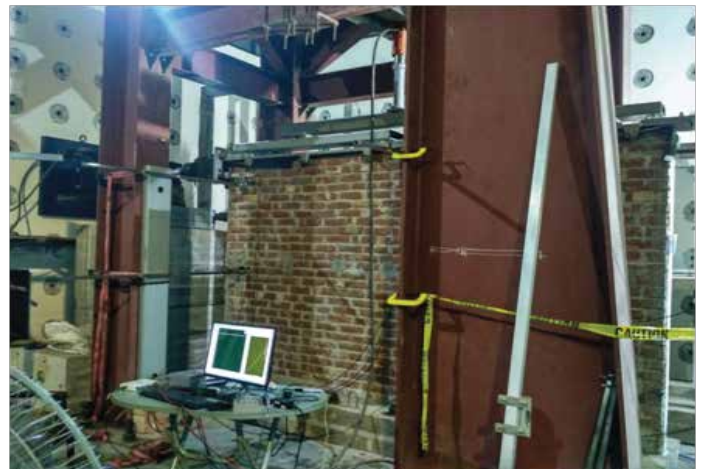
Masonry Wall under Test Setup
