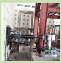
BUET-JIDPUS is conduction a research project in association with Military Institute of Science and Technology (MIST). The primary objective of this research is to investigate the seismic behavior of hybrid concrete column reinforced with different configuration of smart longitudinal reinforcing materials under quasi static cyclic loading test. The study focuses on further expanding the investigation to compare their performance with that of non-hybrid square reinforced
