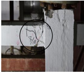
Figure 22. Crack Pattern at Beam-Column Joint
