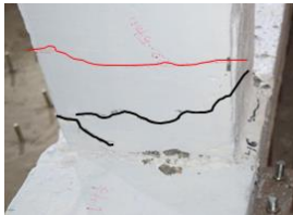
Figure 16. Crack Pattern at Beam-Column Joint
