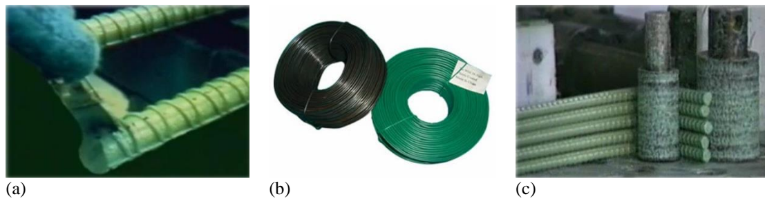
Figure 2. Precautions taken during fabrication. a) Cut ends being repaired with epoxy, b) Coated tie wires and c) Nylon collared mandrel.
