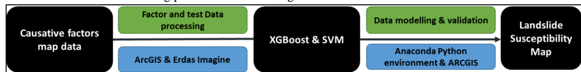
Figure 2. Working process flow of Landslide Susceptibility Mapping
