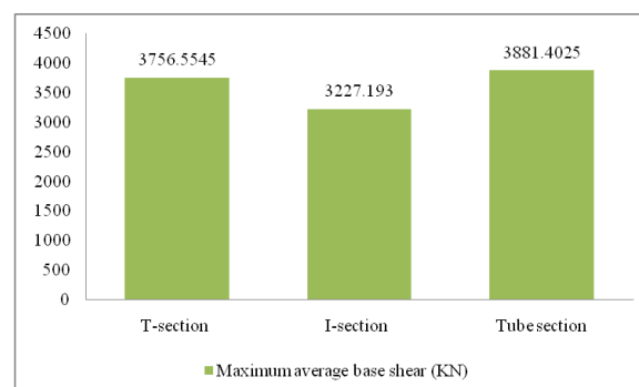
Figure 11. Maximum average base shear considering three section types for ZX bracing.
