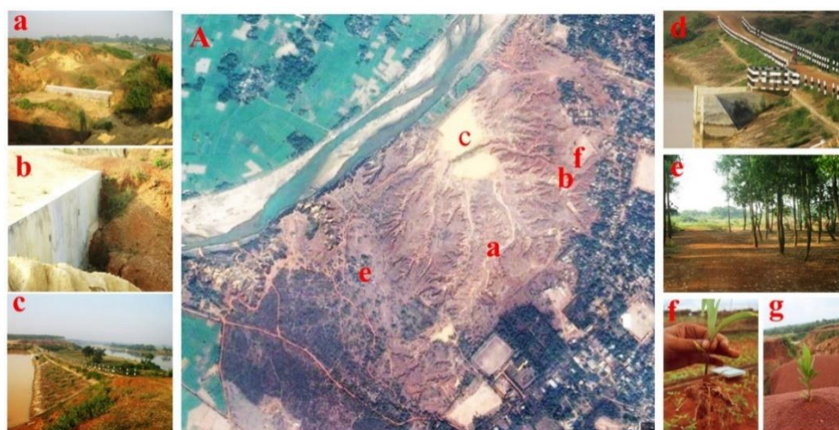
Figure 10. Badland management strategies. Badland area (A), Small checkdam on wide gully channel (a), Checkdam on narrow gully channel (b), Bigdam between at river side (c), Bigdam with lock gate, water storing and water storing pond (d), Previous afforestation project area (e), Plant root developed on geotextile (f), Plantation on the gully head (g)
