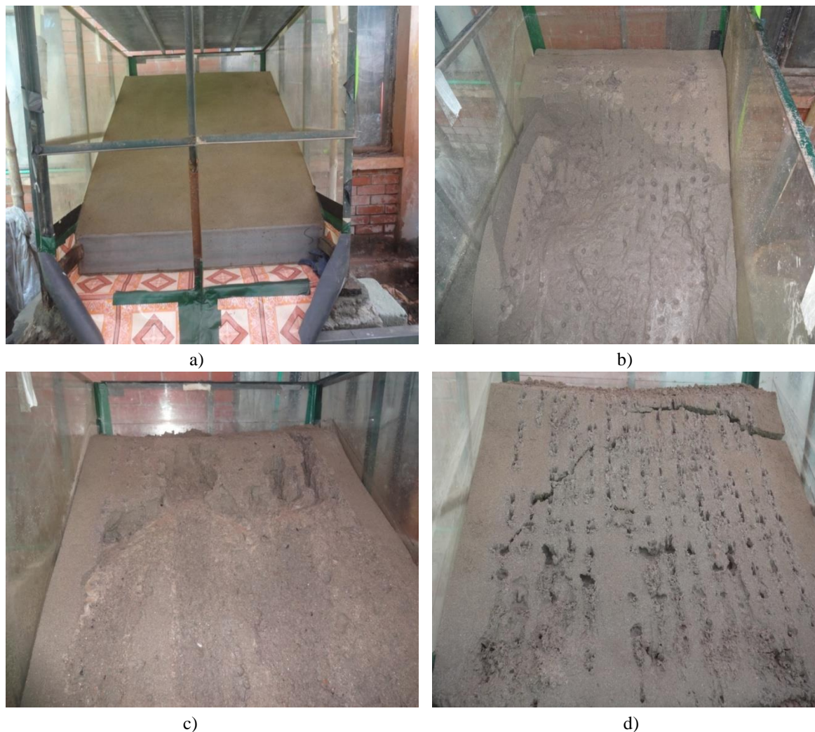
Figure 2: a) Condition of slope for bare soil before rainfall b) Failure state of bare soil slope c) Condition of slope of 500 gsm JGT covered soil after four hours rainfall d) Condition of slope of 700 gsm JGT covered soil after four hours rainfall
