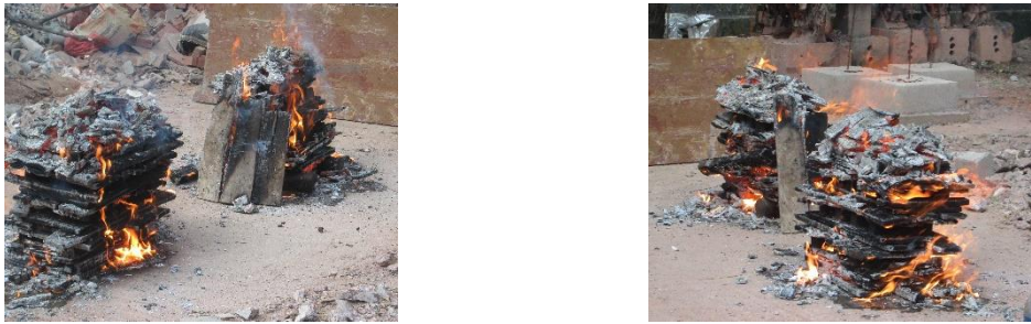
Figure 1. Burning of cement mortar samples under controlled temperature.
