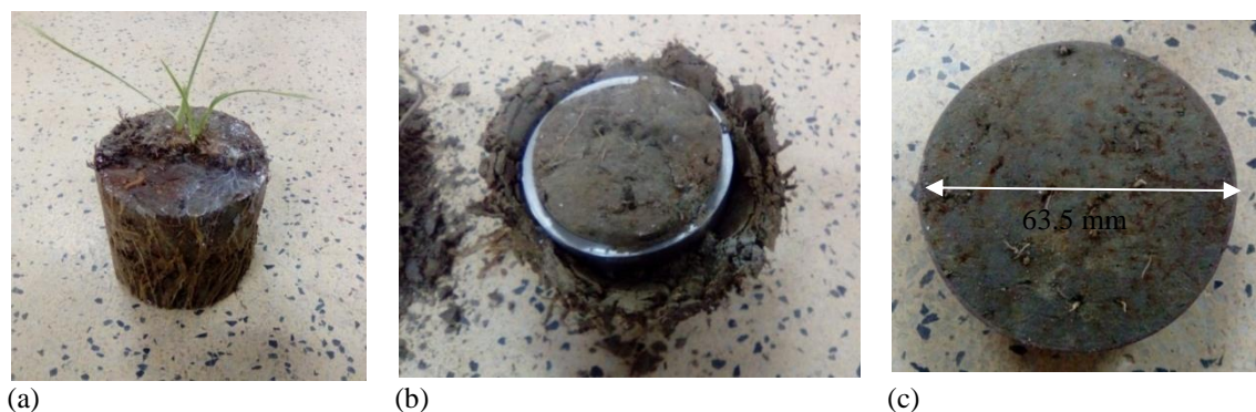
Figure 2. Steps of sample preparation (a) Soil retrieved from pipe, (b) Collection of 62.5 mm dia specimen from 75 dia soil sample, (c) Specimen in probing ring
