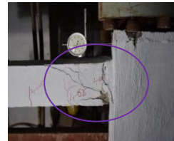
Figure 18. Crack Pattern at Column-Base beam Joint
