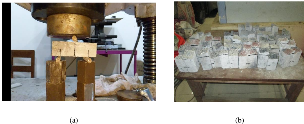
Figure 3. The test procedure for determining the flexural strength of cement mortars. (a) Test setup, (b) Samples after testing
