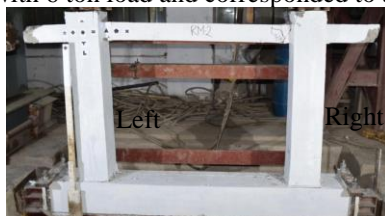
Figure 20. Retrofitted specimen-2 under Hydraulic testing Machine
