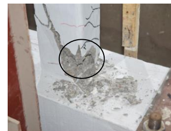
Figure 12. Failure cracks in column- base beam joint at the left column
